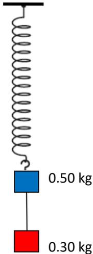
Before the string is cut the tension in the spring is 8.0 N and so the extension is  $x = \frac{8.0}{162} = 4.94 \text{ cm}$ . The new equilibrium position has the spring extended by  $x = \frac{5.0}{162} = 3.09 \text{ cm}$ . The displacement at  $t = 0$  when the string is cut is then  $x = 4.94 - 3.09 = 1.85 \text{ cm}$ . This will be the amplitude of oscillations  $x_0$ .
